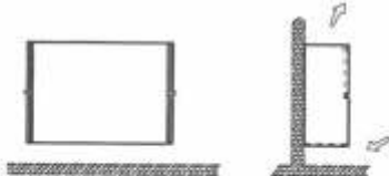
IV - Version hidden vertical mounting with lower suction
